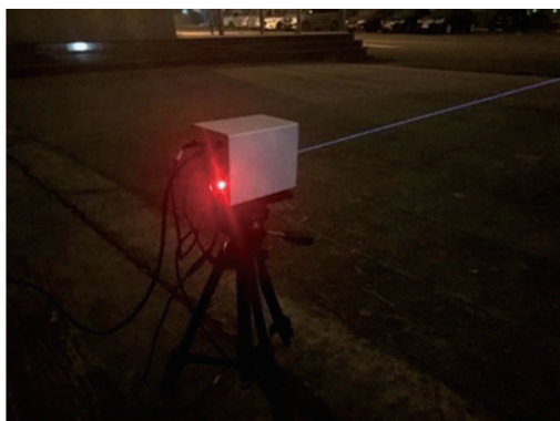
图 4 便携式无组织排放颗粒物测量仪器实物图 Fig. 4 Photograph of portable measuring device for fugitive-dust-emission particulate
