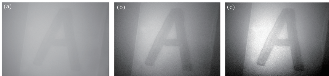
图 7 玻璃纤维板成像对比。(a)预处理强度图像;(b)传统水下偏振差分成像模型的复原图像;(c)改进后的模型的复原图像 Fig. 7 Comparison of glass fiber board imaging. (a) Pre-processed intensity image; (b) image restored by conventional underwater polarization difference imaging model; (c) image restored by improved model
