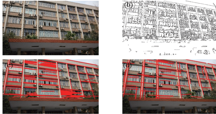
图 8 建筑物图像检测结果比较。(a)原图;(b) Canny 边界;(c) PPHT 结果;(d)本文算法结果 Fig. 8 Comparison of a building image detection results. (a) Original image; (b) Canny edge; (c) PPHT results; (d) our algorithm results
