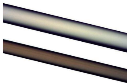
图 1 PbSe-QDF 与普通 SiO 2 单模光纤的对比 Fig. 1 Comparison between PbSe-QDF and conventional SiO 2 single mode fiber
