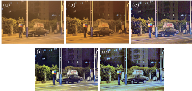
图 11 不同方法对 Street 去雾结果。(a) Street 图;(b)文献[7]算法;(c)文献[12]算法;(d)文献[14]算法;(e)本文算法 Fig. 11 Dehazed results of different methods for Street. (a) Street image; (b) result of Ref. [7] method; (c) result of Ref. [12] method; (d) result of Ref. [14] method; (e) result of proposed method
