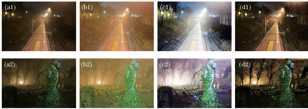
图 7 不同方法的去雾结果。(a1)(a2)输入夜间图像;(b1)(b2) Retinex 算法;(c1)(c2)直方图均衡化;(d1)(d2)本文算法 Fig. 7 Dehazed results of different methods. (a1)(a2) Input nighttime images; (b1)(b2) results of Retinex method; (c1)(c2) results of histogram equalization method; (d1)(d2) results of proposed method
