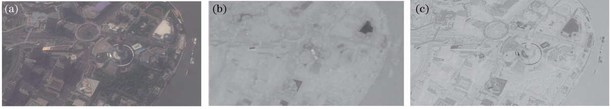
图 1 雾化图像及其透射率分布图。(a) 原图; (b) 文献[2]方法估计透射率图; (c) 本文方法获取透射率图 Fig. 1 Hazed image and its transmission distributions. (a) Original image; (b) estimated transmission map by Ref. [2] method; (c) obtained transmission map by proposed method
