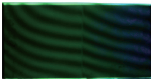
图 12 拼接光栅形成的干涉条纹 Fig. 12 Interference fringe of the tiled-grating
