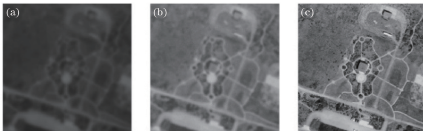
图9 局部放大图像对比。(a) V=15\text{ km} , \theta=80^\circ 下的图像;(b) 自动调光后的图像;(c) WorldView-2原图像 Fig.9 Contrast of partial enlarged images. (a) Image at the condition of V=15\text{ km} , \theta=80^\circ ; (b) image processed by adaptive exposure; (c) original image of WorldView-2
