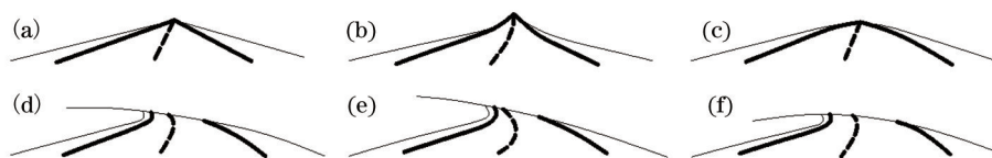
图 1 基本道路模型。(a) 纵向线性斜坡; (b) 凹线; (c) 凸线; (d) 纵向非线性斜坡; (e) 凹曲线; (f) 凸曲线 Fig.1 Basic models of the road. (a) Longitudinal linear slope; (b) concave line; (c) convex line; (d) longitudinal non-linear slope; (e) concave curve; (f) convex curve
