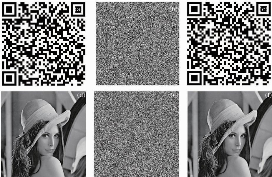
图 4 算法加解密效果图。(a)和(d)为二维码和 Lena 原图; (b)和(e)为相应的加密图像; (c)和(f)为相应的解密图像 Fig. 4 Performance of the proposed system. (a) Original twodim; (b) cipher image of Fig. 4(a); (c) decrypted image of Fig. 4(b); (d) original Lena; (e) cipher image of Fig. 4(d); (f) decrypted image of fig. 4(e)
