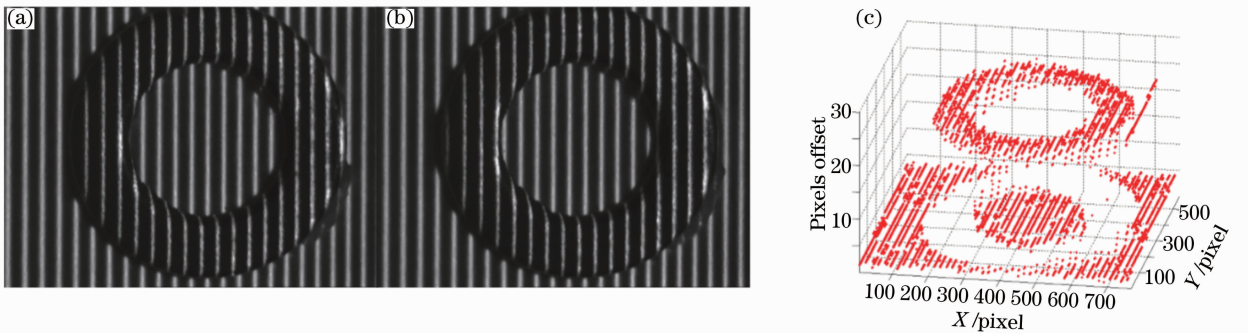
图 10 窄脉宽调制的条纹图及条纹中心提取分析。(a)和(b)为采集的相位差为 \pi 的条纹;(c)光条中心偏移量分布 Fig. 10 Narrow pulse-width modulation fringe patterns and the center extraction analysis. (a) and (b) are captured fringes with \pi phase shift; (c) pixels offset distribution of the fringe center
