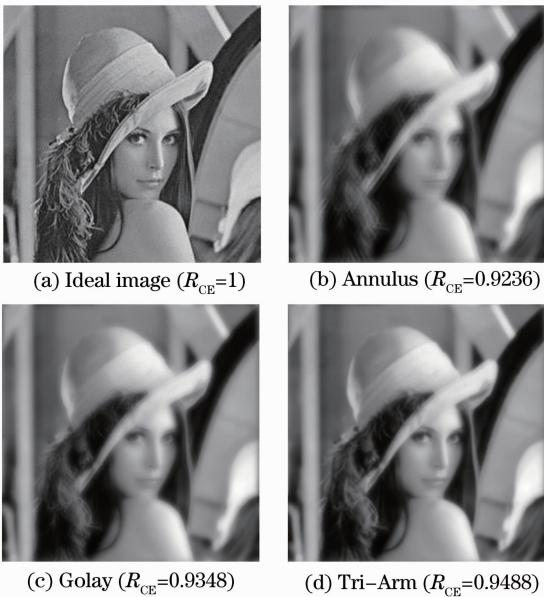
图 4 F=0.3 时三种阵列直接成像结果 Fig. 4 Direct imaging results of three arrays when F=0.3
