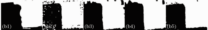
(b) binarization of figure 6(a), from left to right threshold for: 10 (b1), 62 (b2), 68 (b3), 78 (b4), 108 (b5)
