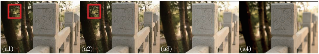
(a) from left to right: image focus on foreground (a1), image focus on background (a2), SLR cameraeffect (a3), depth of field simulation (a4)
