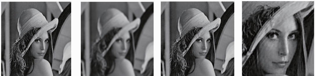
(a) original image (b) noisy and blurred image (c) recovered image (d) facial detail of recovered image
