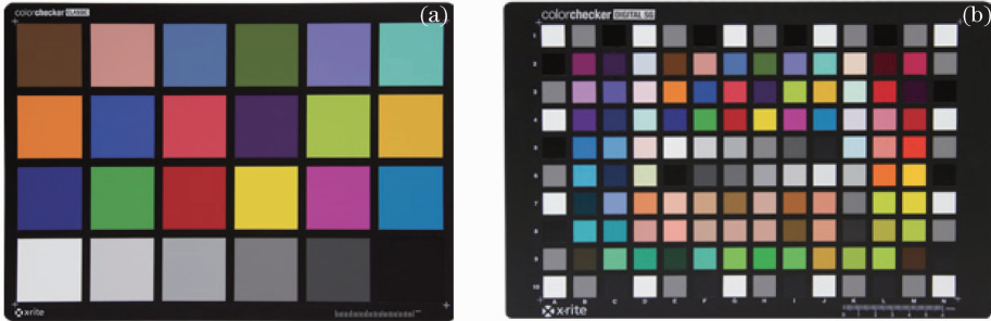
图 1 (a) ColorChecker Classic 24 色迷你小色卡; (b) ColorChecker SG 色卡 Fig. 1 (a) Colorcheck 24 patch dassic target; (b) ColorChecker SG color card
