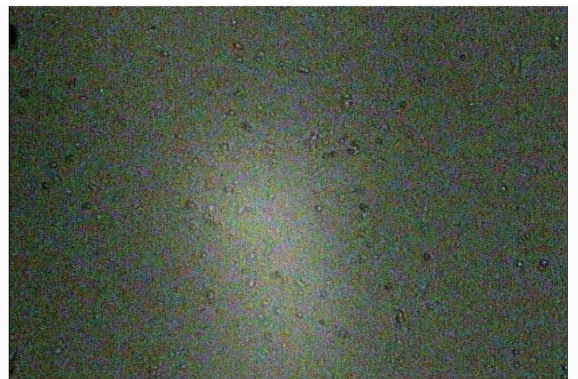
图 7 束流为 50 mA 时膜层表面质量 Fig. 7 Film surface quality with the ion beam current of 50 mA
