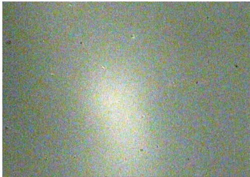
图 6 束流为 25 mA 时膜层表面质量 Fig. 6 Film surface quality with the ion beam current of 25 mA
