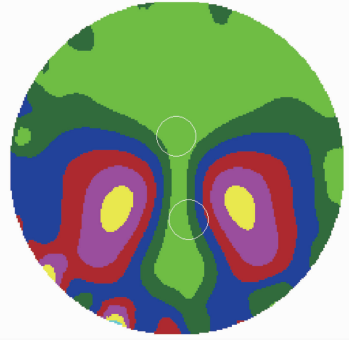
图 10 优化后渐进多焦点眼镜片等散光度图 Fig. 10 Cylinder of manufactured optimized lens
