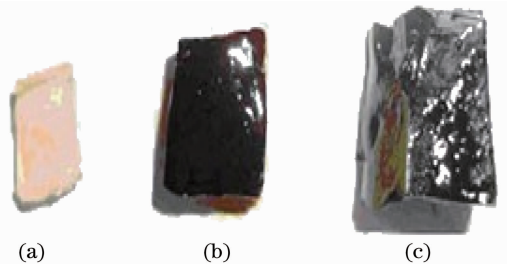
图 4 聚丙烯酸/CTAB-聚吡咯的数码照片图。(a)聚丙烯酸/CTAB 凝胶;(b)聚丙烯酸/CTAB 凝胶电解质;(c)聚丙烯酸/CTAB-PPy 凝胶电解质 Fig. 4 Digital photographs of (a) poly(acrylic acid-g-CTAB) polymer, (b) poly(acrylic acid-g-CTAB) gel electrolyte and (c) poly(acrylic acid-g-CTAB)-polypyrrole gel electrolyte
