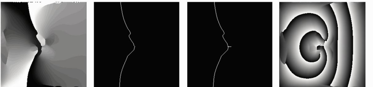
(a) angle distributio after 2D AWT (b) discontinuity border in the horizontal direction (c) discontinuity border in the vertical direction (d) phase without sign ambiguity
