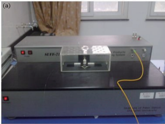
图 2 (a)实验室所用的熔融拉锥机；(b)小模场直径 PCF2 实验效果图；(c)大模场直径 PCF3 实验效果图 Fig. 2 (a) Picture of fusion taper rig; (b) schematic longitudinal cross section of PCF2; (c) schematic longitudinal cross section of PCF3
