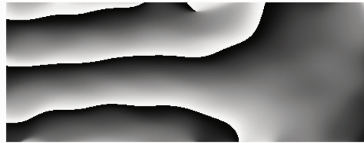
图 11 激光器 A 照射物体变形包络相位图 Fig. 11 Wrapped phase distribution of deformation when the object is illuminated by laser A
