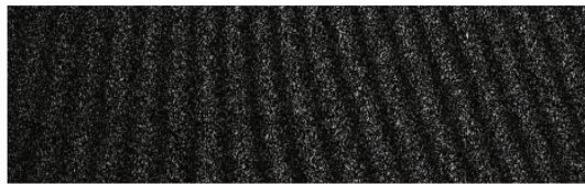
图 9 激光器 B 照射试件变形后受调制载波条纹 Fig. 9 Modulated carrier fringe after deformation when the object is illuminated by laser B
