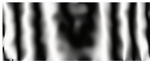
图 15 面内位移垂直分量( v 场)的条纹图 Fig. 15 In-plane displacement fringe of field v in vertical direction
