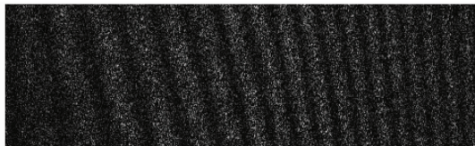
图 10 激光器 C 照射试件变形后受调制载波条纹 Fig. 10 Modulated carrier fringe after deformation when the object is illuminated by laser C
