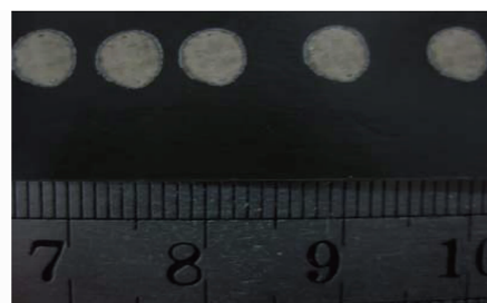
图1 未用光纤耦合的钬激光脉冲光斑图 Fig. 1 Thermal images of the holmium laser spot without fiber coupler
