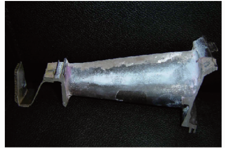
图 6 四级导向器分解叶片打磨后恢复形状和尺寸 Fig. 6 Figure and size of the fourth oriented implement after polishing
