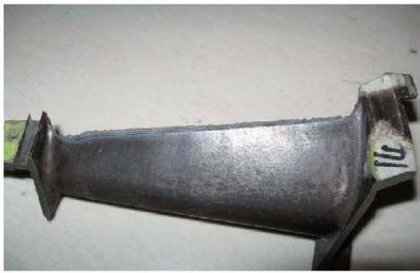
图 5 修复后的四级导向器分解叶片(未打磨) Fig. 5 Decompose lamina of the fourth oriented implement after repair(before polishing)
