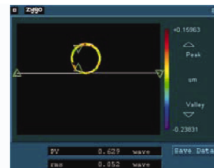
图 6 补偿器法全口径实验测量结果 Fig. 6 Result of full aperture experimental by compensator
