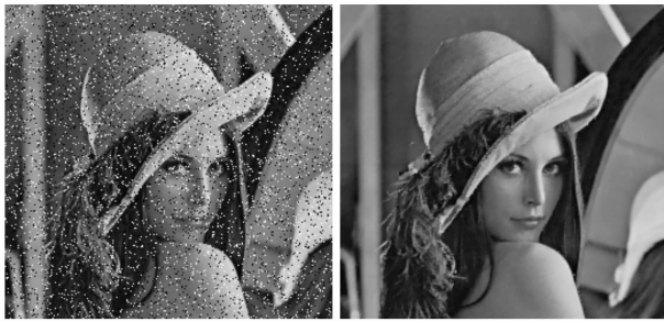
图 3 10%椒盐噪声污染的 Lena 图像及滤波后结果 Fig.3 Lena iamge corrupted by 10% salt & pepper noise and the filtering result
