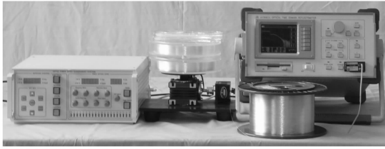
图 6 并联双环瑞利后向散射式光纤陀螺的实验装置 Fig.6 Experimental setup of the two-ring combined in parallel Rayleigh back scattering gyroscope
