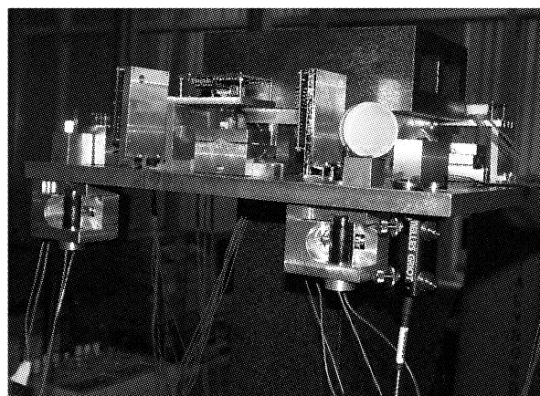
Fig. 8 The photo of the laser collimation system. 1: single-mode fiber; 2: beam two-dimensional moving system; 3: fiber coupling system; 4: parallel movement mirror; 5: the measurement for displacement drift; 7: rotating angle reflector; 8: beam two-dimensional rotating system
