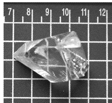
Fig. 1 As-grown crystal of BIBO
