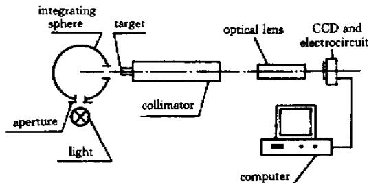
Fig. 2 Schematic diagram of MTF testing system
