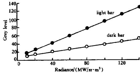
Fig. 3 CCD response to target bar
