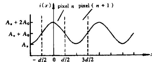
Fig. 1 Schematic diagram of spatial relation between target image function and pixels in Nyquist frequency
