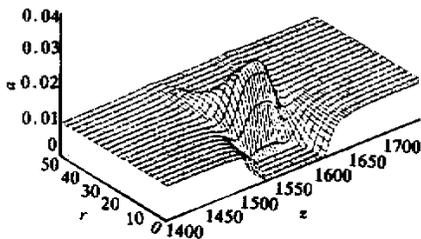
Fig. 5 The 2D distribution of electron density, where  $a_0 = 2$ ,  $Zn_i = 0.01$ ,  $r_0 = 100$  and  $r_s = 40$
