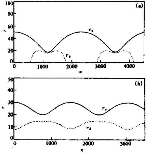
Fig. 3 The spot size  $r_s$  (solid curve) and the size of the cavity  $r_d$  (dotted line) versus  $z$ , where  $a_0 = 2, Zn_i = 0.01, r_0 = 100$  and  $r_s = 40$
