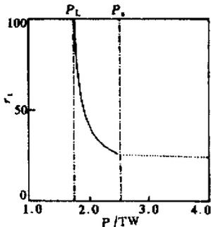
Fig. 2 The dependence of laser power  $P$  and the size of self-guiding  $r_t$  for  $Zn_i = 0.01$
