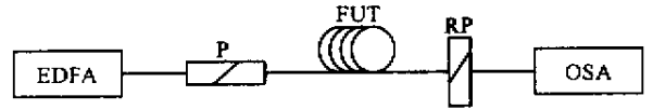
Fig.6 Measurement setup. P: polarizer; FUT: fiber under test; RP: rotatable polarizer; OSA: optical spectrum analyzer
