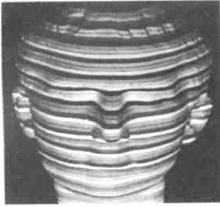
Fig. 1 The image of color-coded grating of 3-D measurement
