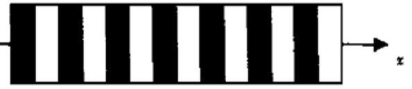
Fig. 1 The simple model of multilayer. The black part represent the absorption, and the white part is the spacing
