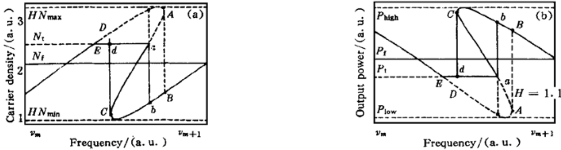
Fig. 2 The hysteresis loop of an ECLD (calculated for H = 1.1 ). (a) The N - \nu hysteresis loop, (b) The P - \nu hysteresis loop
