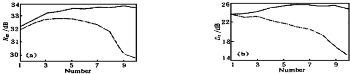
Fig. 3 Computer simulation showing R_{\text{SN}} and D_r changing according to the period number of cosine function used
