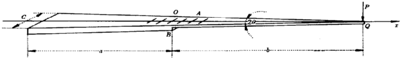
Fig. 1 Schematic diagram of the designed cantilever beam
