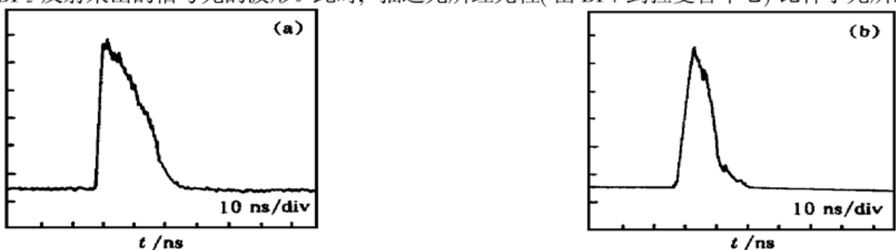
Fig. 4 The Stokes waveform without pump (a) and with pump (b). The pump energy is 150 mJ and the pulse duration is 22 ns. The seed-Stokes has energy of 0.1 mJ and pulse duration of 16 ns. The pressure of hydrogen in the Raman cell is 0.91 MPa
