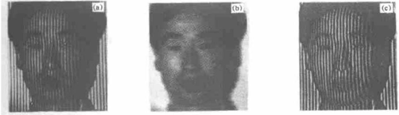
Fig. 6 Example of relative distorted grating image created by wavelet transform. (a) Original modulated grating image; (b) Background image by wavelet transform; (c) Relative distorted grating image.
