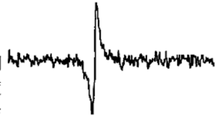
Fig. 4 The lineshape of modulation transfer spectrum
