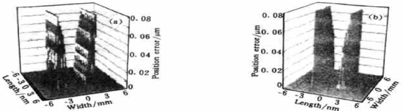
Fig. 6 Theoretical error distribution on the sensitive area of PSD caused by diffraction. (a) Error profile in x direction, (b) Error profile in y direction
