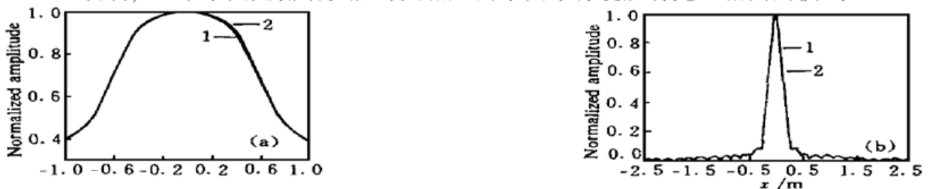
Fig. 2 Amplitude distribution of the lowest-order mode. (a) On the total reflector of each resonator; (b) At a 200 m distance from the grating or output mirror. 1: a plane mirror-grating resonator; 2: a parallel plane mirror resonator
