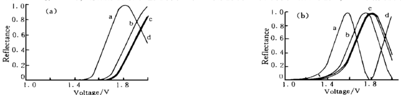
Fig. 10 Relative intensity of output light from LCLV versus voltage across the LC for different anchoring energy. (a) \theta_{00} = 0^\circ , (b) \theta_{00} = 3^\circ . a: C = 5 \times 10^{-5} \text{ J/m}^2 , b: C = 2 \times 10^{-4} \text{ J/m}^2 , c: C = 1 \times 10^{-3} \text{ J/m}^2 , d: C = \text{infinity}
