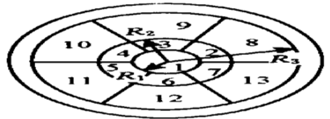
Fig. 2 Electrode pattern of 13-segment bimorph deformable mirror
