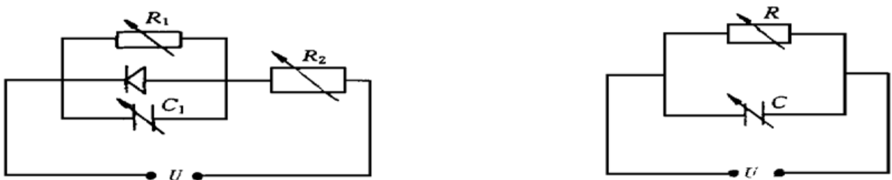
Fig. 3 Equivalent circuit of photo-sensor
