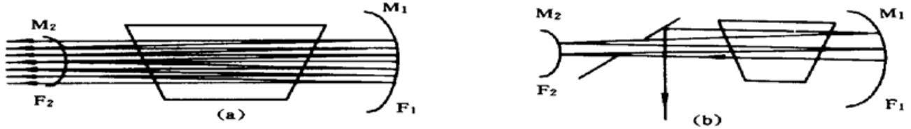
Fig. 8 The schematic diagram of the propagation of the laser in the unstable resonator. (a) The confocal positive-branch unstable resonator, (b) The output of the 5-pass
