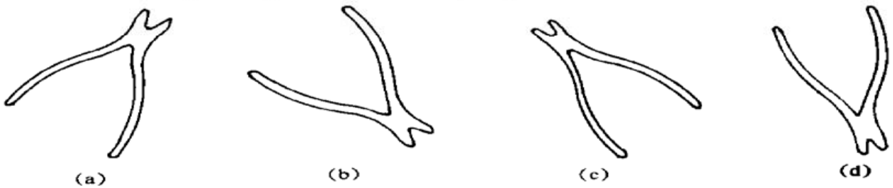
Fig. 1 Procedure for obtaining boundary image. (a) Digitized image of pliers. (b) Edge image extracted using Sobel operator. (c) Boundary image
