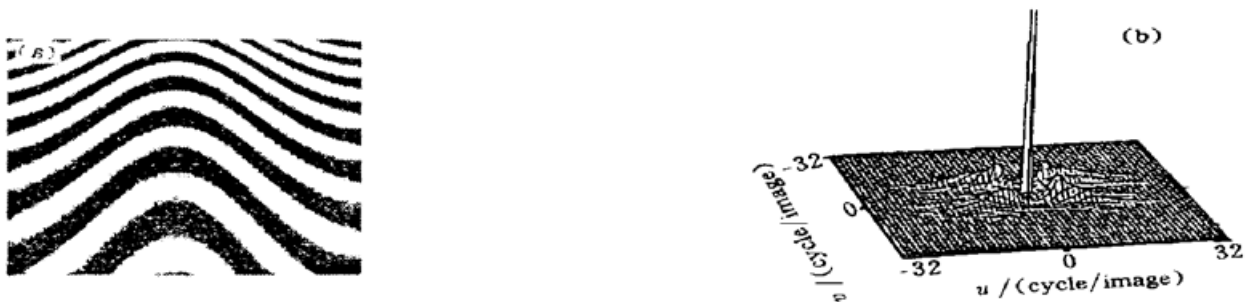
Fig. 3 (a) A simulated interferogram with gradually increasing reference frequency, (b) Fourier frequency spectrum of (a)
