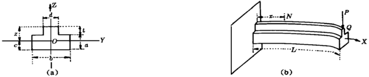
Fig. 1 Schematic of \perp -shaped bent cantilever beam. (a) Cross-section of the cantilever, (b) Deformation of the bent cantilever
