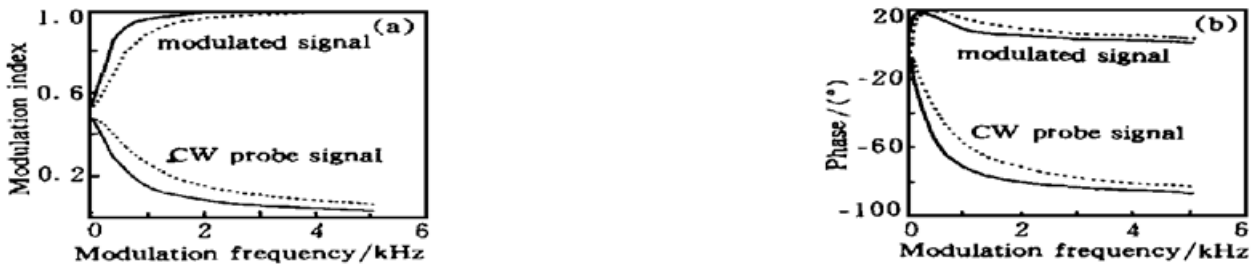
Fig. 1 Frequency response at small-signal modulation. Input power is - 10 dBm (solid line) and - 20 dBm (dashed line). (a) Amplitude, (b) Phase delay
