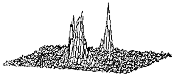
Fig. 6 Spatial distribution of light spots of ordinary ruby laser (left) and of that with SBS phase conjugate mirror (right)
